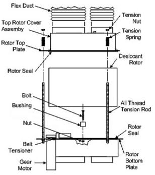
Figure 10 - Rotor Assembly Parts
