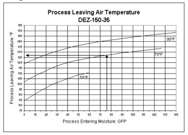
**NOTE**: Process air outlet temperatures as shown are maximum values at standard full rated heater output. The actual process outlet temperature will be lower when the heater output is below full rated output. This condition will occur during heater modulation cycles due to partial loading of the dehumidifier.
