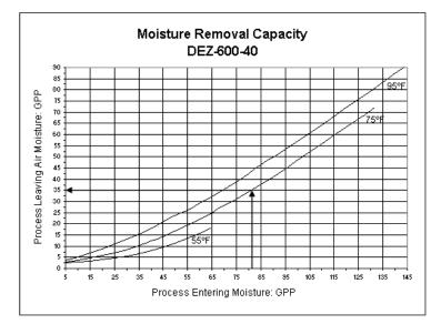
**NOTE:** Process air outlet temperatures as shown are maximum values at standard full rated heater output. The actual process outlet temperature will be lower when the heater output is below full rated output. This condition will occur during heater modulation cycles due to partial loading of the dehumidifier.
