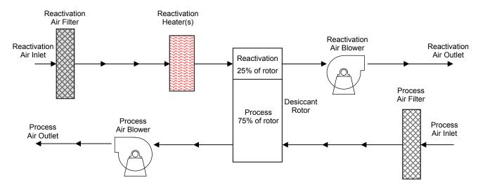
Figure 2 - General Theory of Operation Diagram
