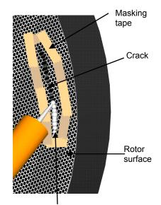
Apply silicone using an upward motion to push silicone into crack
