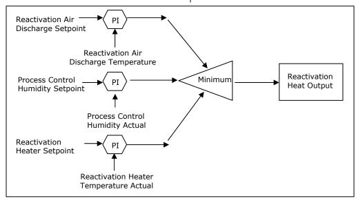
Figure 4 - Proportional (Trac) Control Diagram
