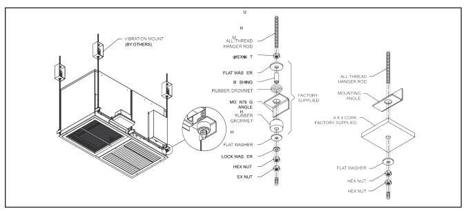
Figure 6. Typical Installation
