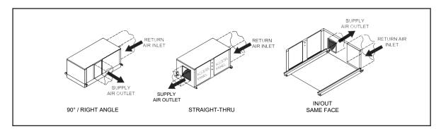
Figure 9. Ducted System Typical Air Patterns
