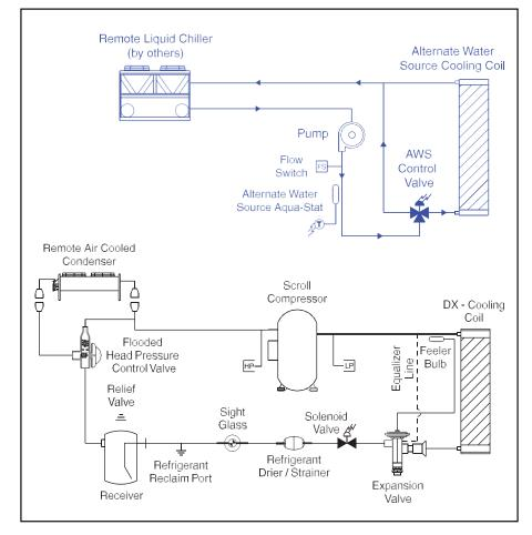
Figure 5. Alternate Water Source Diagram
