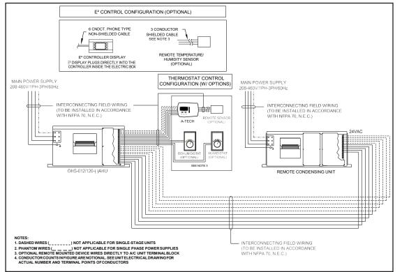
Figure 19. Interconnection Field Wiring Remote Condensing Unit with Dual Compressors
