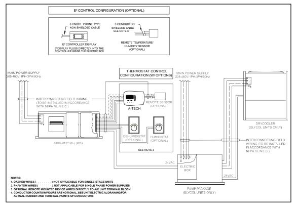
Figure 20. Interconnection Field Wiring Glycol Systems
