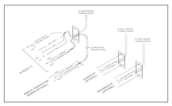
Figure 15. A-Tech 1.1 Control Wiring
