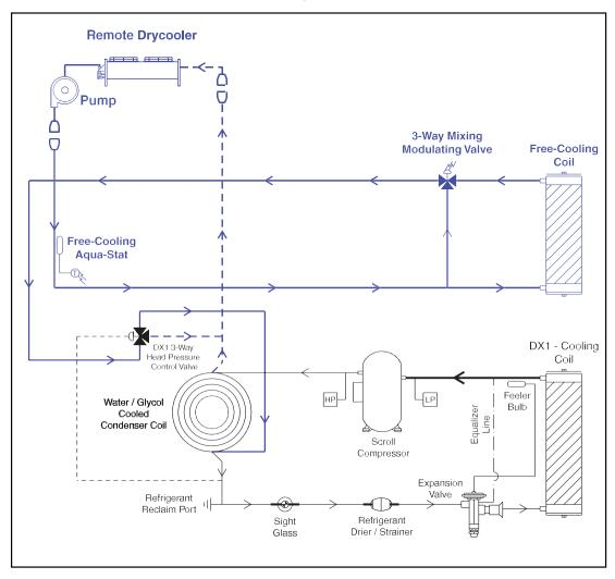
Figure 4. Free Cooling Diagram
