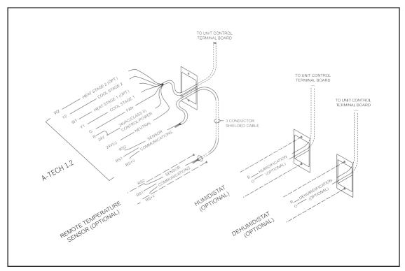
Figure 16. A-Tech 1.2 Control Wiring
