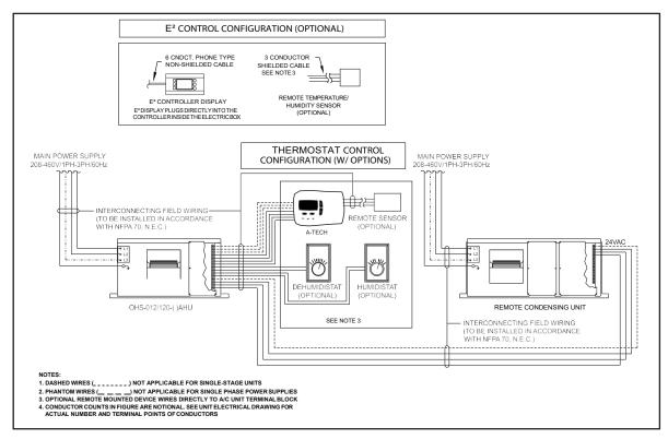
Figure 18. Interconnection Field Wiring Remote Condensing Unit
