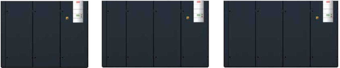
CyberAir 3 air conditioning units in standard door sizes are available as energy or space-saving versions. The seven available sizes range from 950 to 3,350 mm in width. The largest two sizes have a depth of 980 mm.
