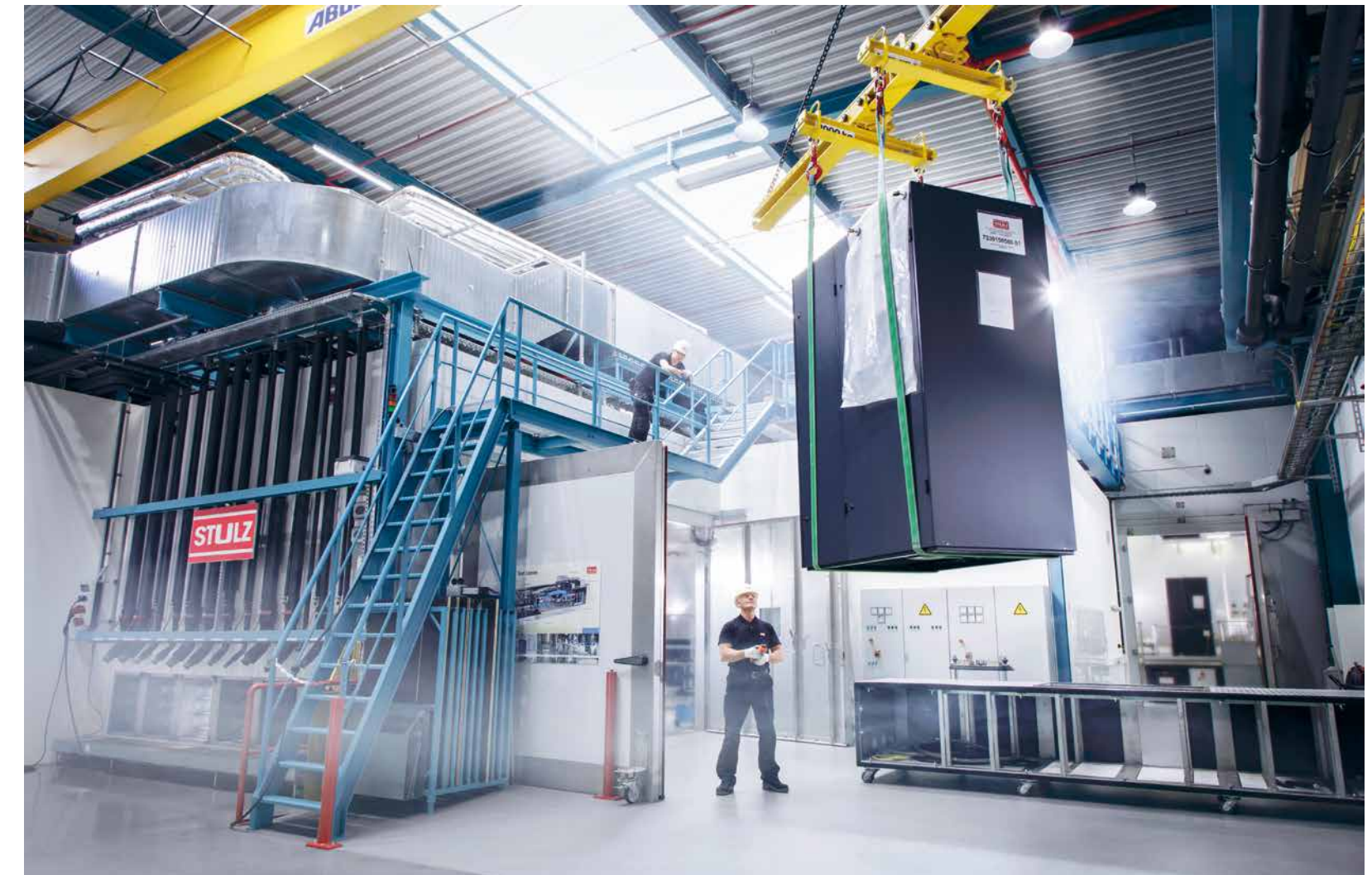
Fig. 1: Over an area of around 700 square meters, STULZ operates one of Europe's most state-of-the-art test facilities for air conditioning technology. The plant boasts two separate climatic chambers and four conditioning systems.
