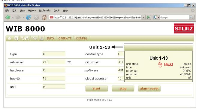
All parameters which are not displayed on a grey background, can be modified by marking the value and typing the new value. The modification will be effective when you confirm it by clicking on the "Send" button.
