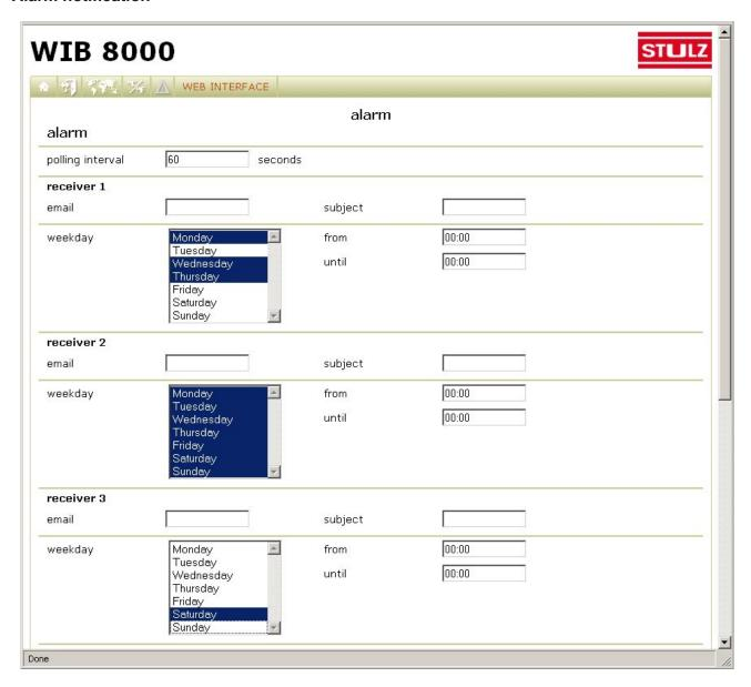
You can enter up to five receivers or time spaces for the notification via e-mail when alarms occur. You can set the days at which this shall happen individually for each receiver (for several days by mouseclick while keeping the Ctrl-key pressed). The time spaces can also be set specifically for each receiver.
