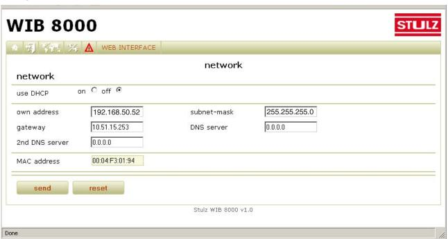
The indication of a DNS address (only IP address possible) is compelling, if server names for other servers (mail, NTP, SNMP Trap) shall be entered instead of their IP addresses.
