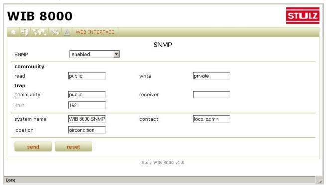
For safety reasons the customer may want to lock the SNMP access. All network modifications are effective only after a reboot of the WIB. You can comfortably reboot the WIB by clicking on the menu item "reboot" in the menu "WEB INTERFACE".
