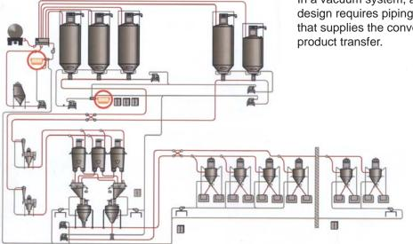
In a vacuum system, a similar approach is employed. Here the design requires piping the vacuum inlet to a plenum or header that supplies the conveying system with dehumidified air for product transfer.
