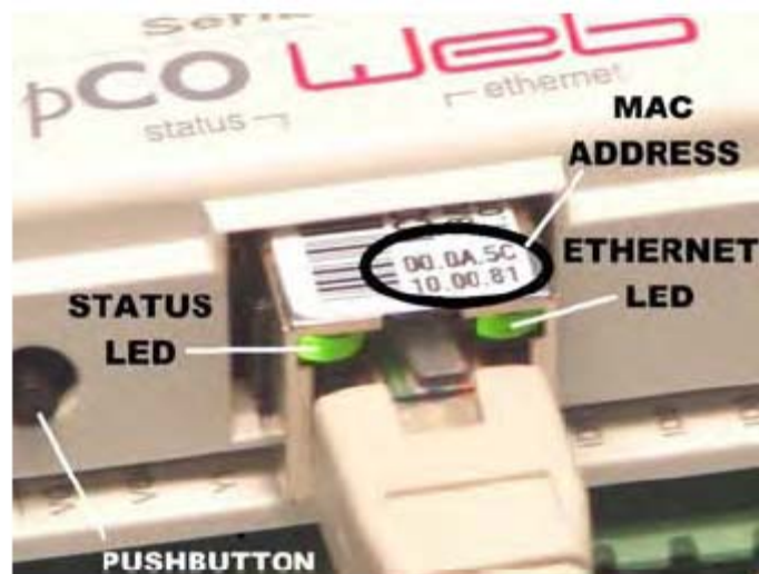
Figure 1.b - MAC address and indicator LEDs
