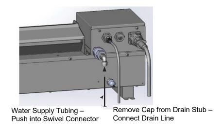
Figure 7. Water Supply and Drain
