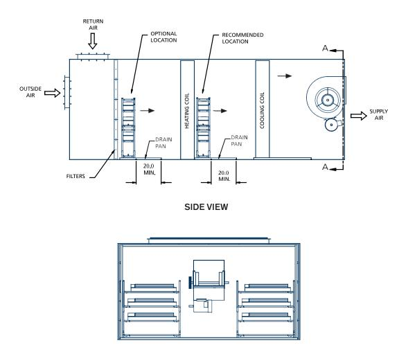
Figure 4. Ultrasonic Humidifier Mounting
