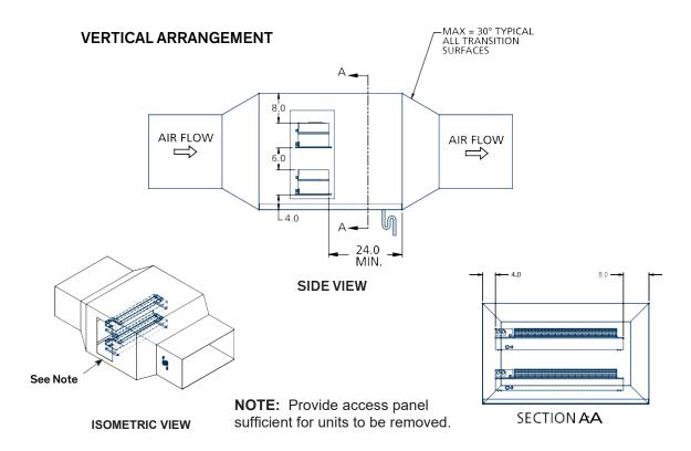
Figure 5. Duct Mounting — Vertical Arrangement
