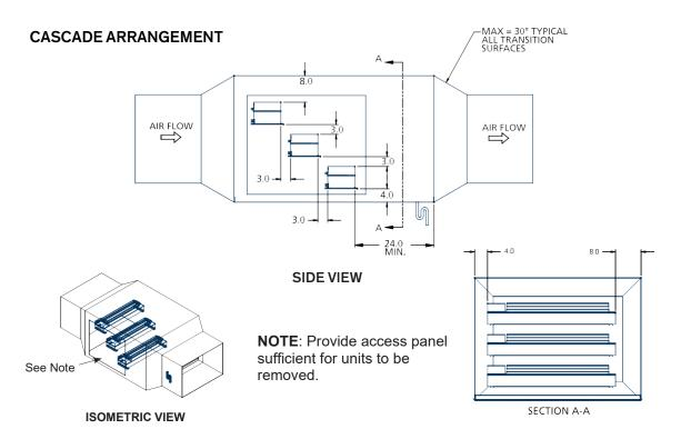
Figure 6. Duct Mounting — Cascade Arrangement
