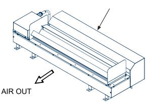
Figure 2. Booster Fan Assembly
