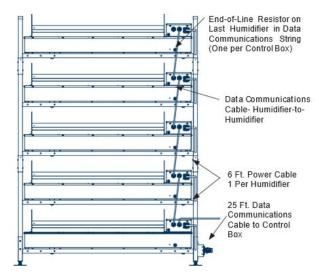
Figure 8. Power and Control Wiring
