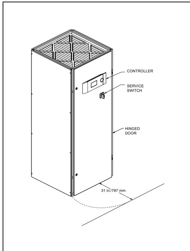
**Figure 5. Recommended Installation Clearance**
