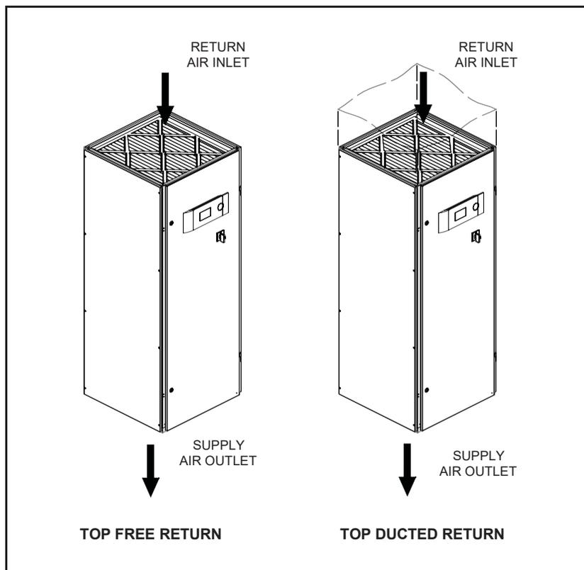
**Figure 7. Downflow Configuration Typical Air Patterns**
