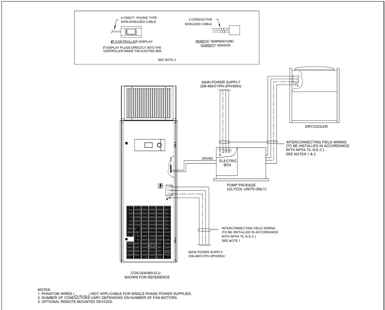
Figure 15. Interconnecting Field Wiring Glycol Systems
