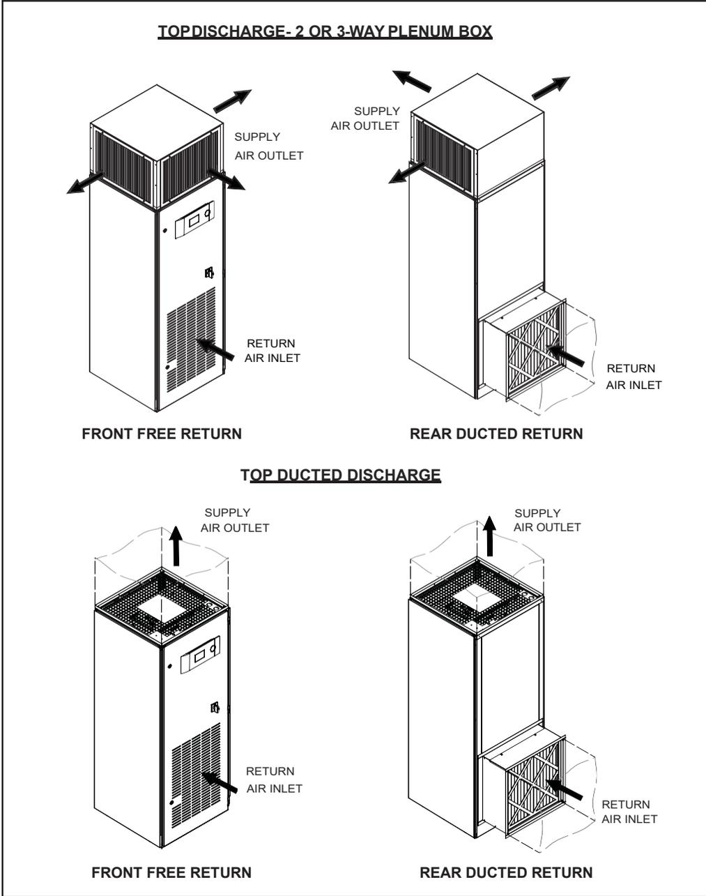
Figure 8. Upflow Configuration Typical Air Patterns
