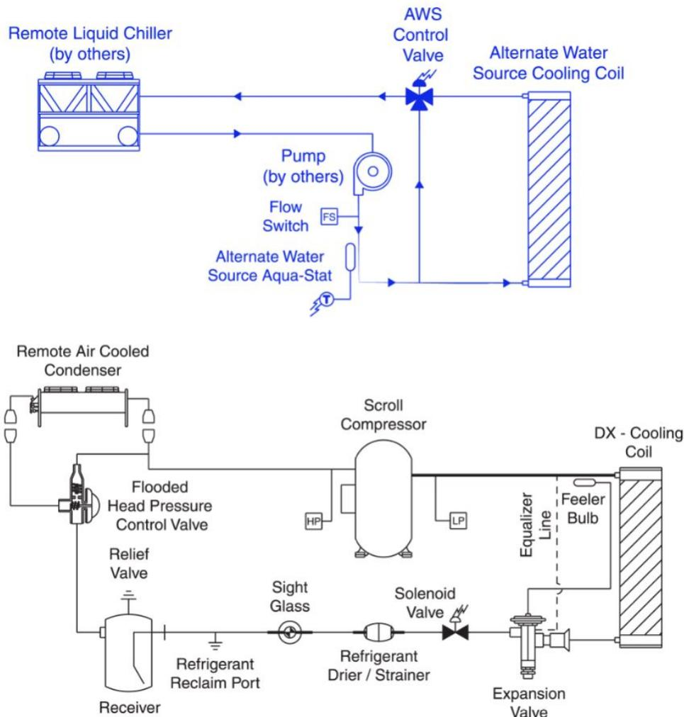
Figure 4. Alternate Water Source Diagram
