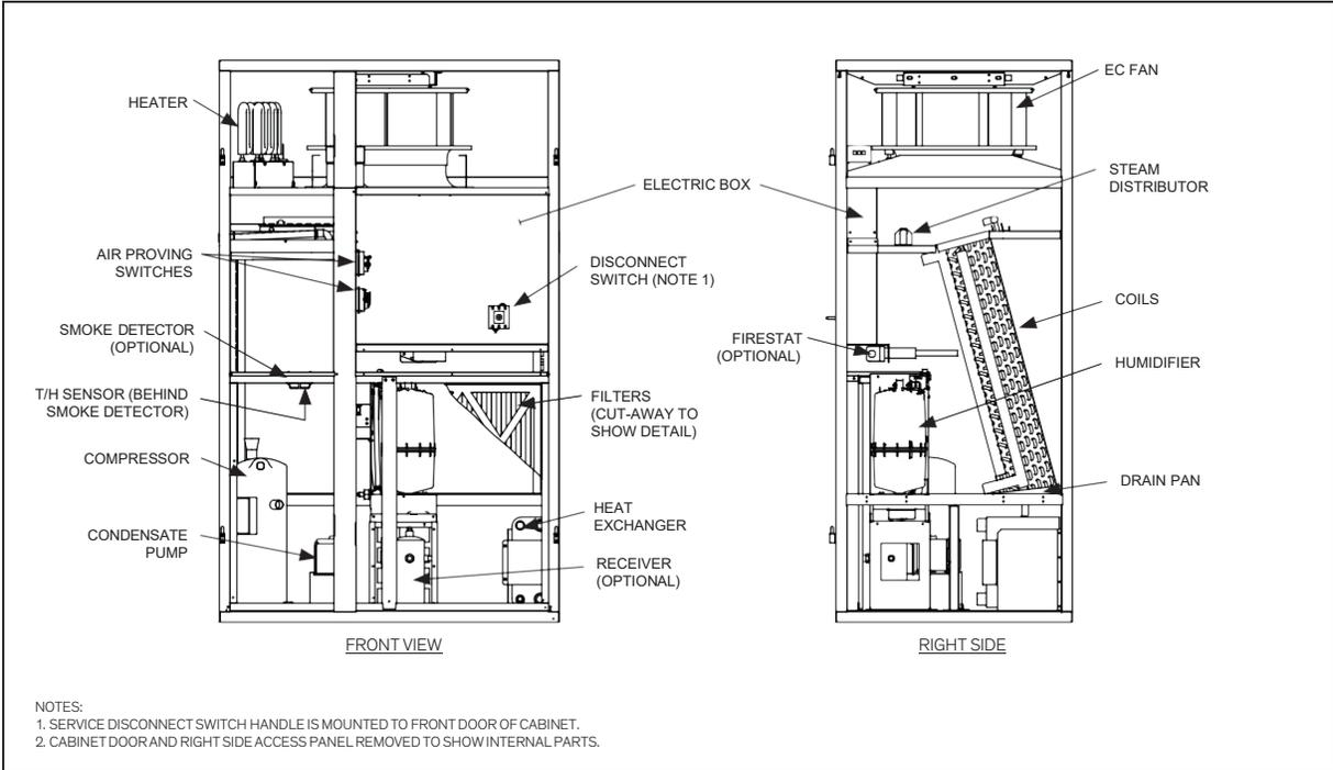
Figure 2. Typical Internal Layout- Upflow Configuration
