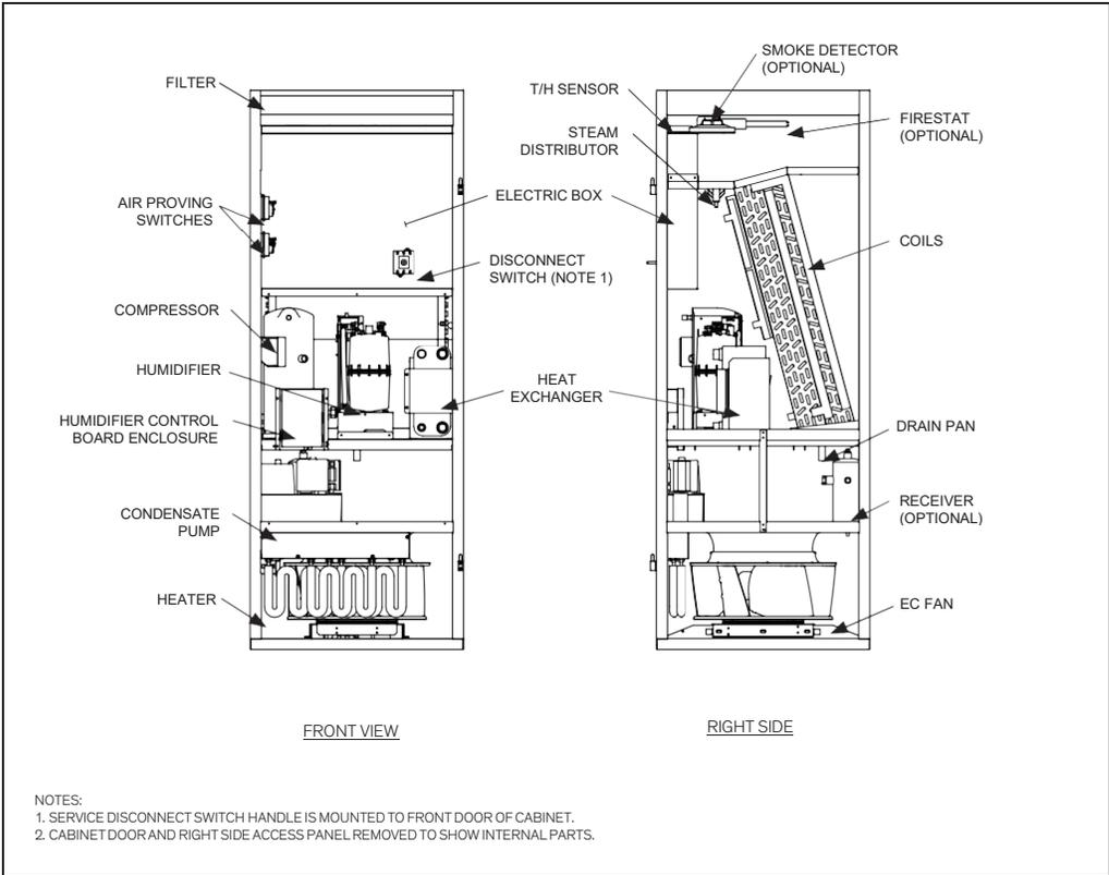
Figure 1. Typical Internal Layout- Downflow Configuration
