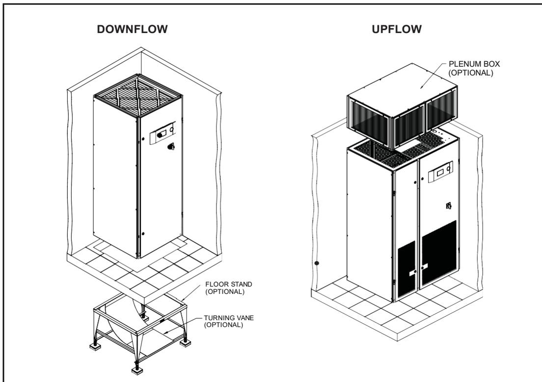
Figure 6. Typical Installation
