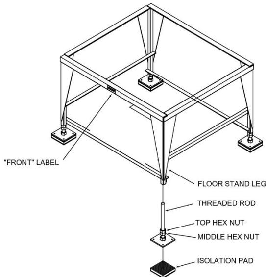
Figure 9. Optional Floor Stand Installation
