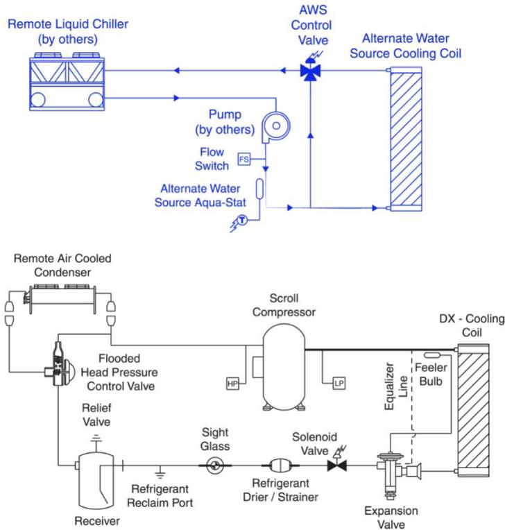
Figure 3. Free Cooling Diagram
