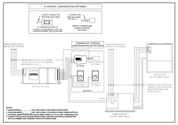
Figure 20. Interconnection Field Wiring Glycol Systems
