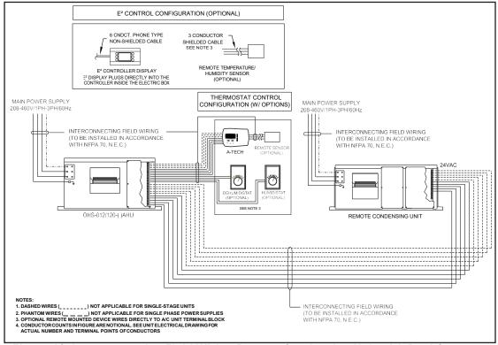
Figure 19. Interconnection Field Wiring Remote Condensing Unit with Dual Compressors
