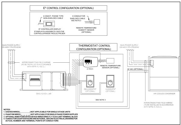
Figure 17. Interconnection Field Wiring Remote Condenser
