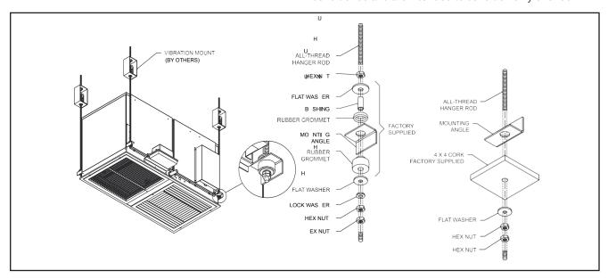
Figure 6. Typical Installation
