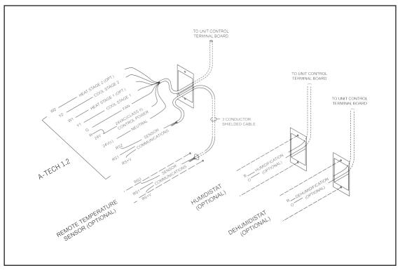
Figure 16. A-Tech 1.2 Control Wiring
