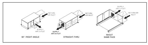
Figure 9. Ducted System Typical Air Patterns
