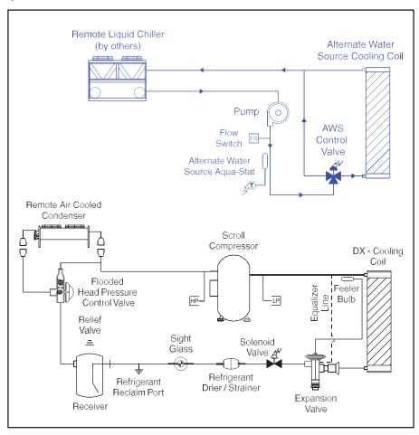
Figure 5. Alternate Water Source Diagram
