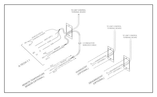
Figure 15. A-Tech 1.1 Control Wiring
