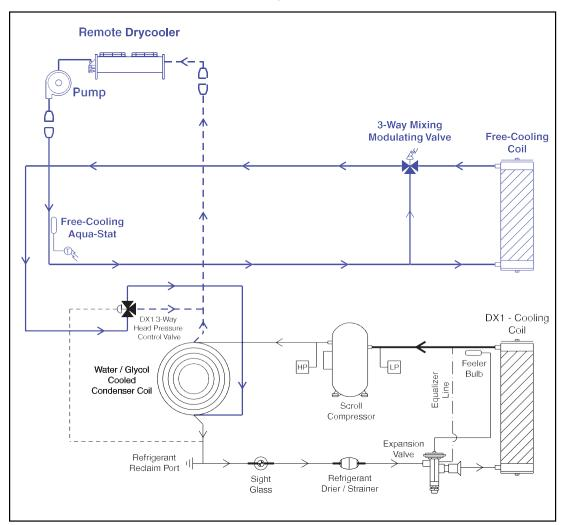
Figure 4. Free Cooling Diagram
