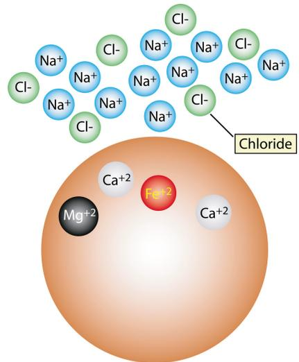
Back flush of salt water through resin to force ion exchange to regenerate resin
