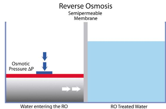
As pressure of the process water is increased, the effectiveness of the RO Plant increases
