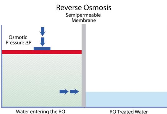
Reverse Osmosis is possible when pressure is applied to the process fluid
