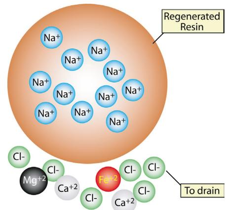
Regenerated resin with hard minerals and chloride drained away
