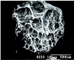
**Figure 5 - Micropores of activated charcoal as seen through 10k magnification**
