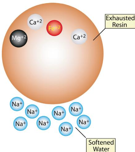
Ion exchange softening water by removal of hard minerals with sodium
