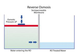
Reverse Osmosis is possible when pressure is applied to the process fluid
