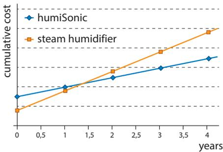
Comparison of total cost between humiSonic and an isothermal humidifier. The higher upfront investment in humiSonic is generally paid back in less than two years.
