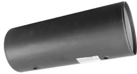
The automatic air vent includes an air separating trap and liquid control baffle to assure unrestricted airflow to the tank and air-free liquid flow from the tank. It also includes a manual vent for adjusting the air volume in the tank. The expansion tank is to be installed at the highest point of the glycol system with the air vent facing down.
